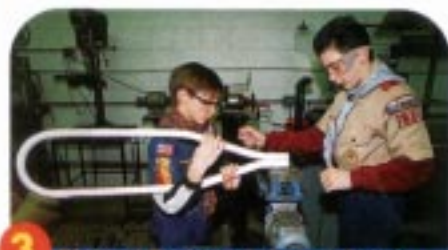
3 Richard Parsons, left, and James Chagon fasten the snowshoe frame's back end with bolts and nuts.
