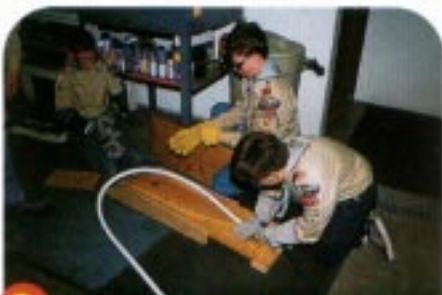
2 The hot sand softens the PVC so that David Newell can fit it in the wooden jig. After the sand cools, the pipe keeps its new shape. Compressed air forces out sand for reheating.
