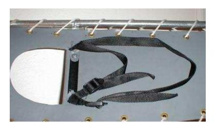
The binding will be attached with two screws that go through the crossbar. Put two marks centered along the width of the crossbar 1/2 inch in from the edges of the foot hole. Drill a hole at each of these marks right through the Hypalon, crossbar, and flap of Hypalon on the bottom. You may wish to enlarge the holes in the hypalon a little bit to allow for some movement.
