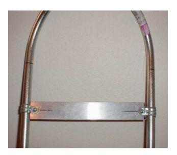
Decide where you want the crossbar to be -- this will be right under the ball of your foot. Measure the distance between the insides of the frame at that point and cut a piece of aluminum strap 1/2 inch shorter than that.
