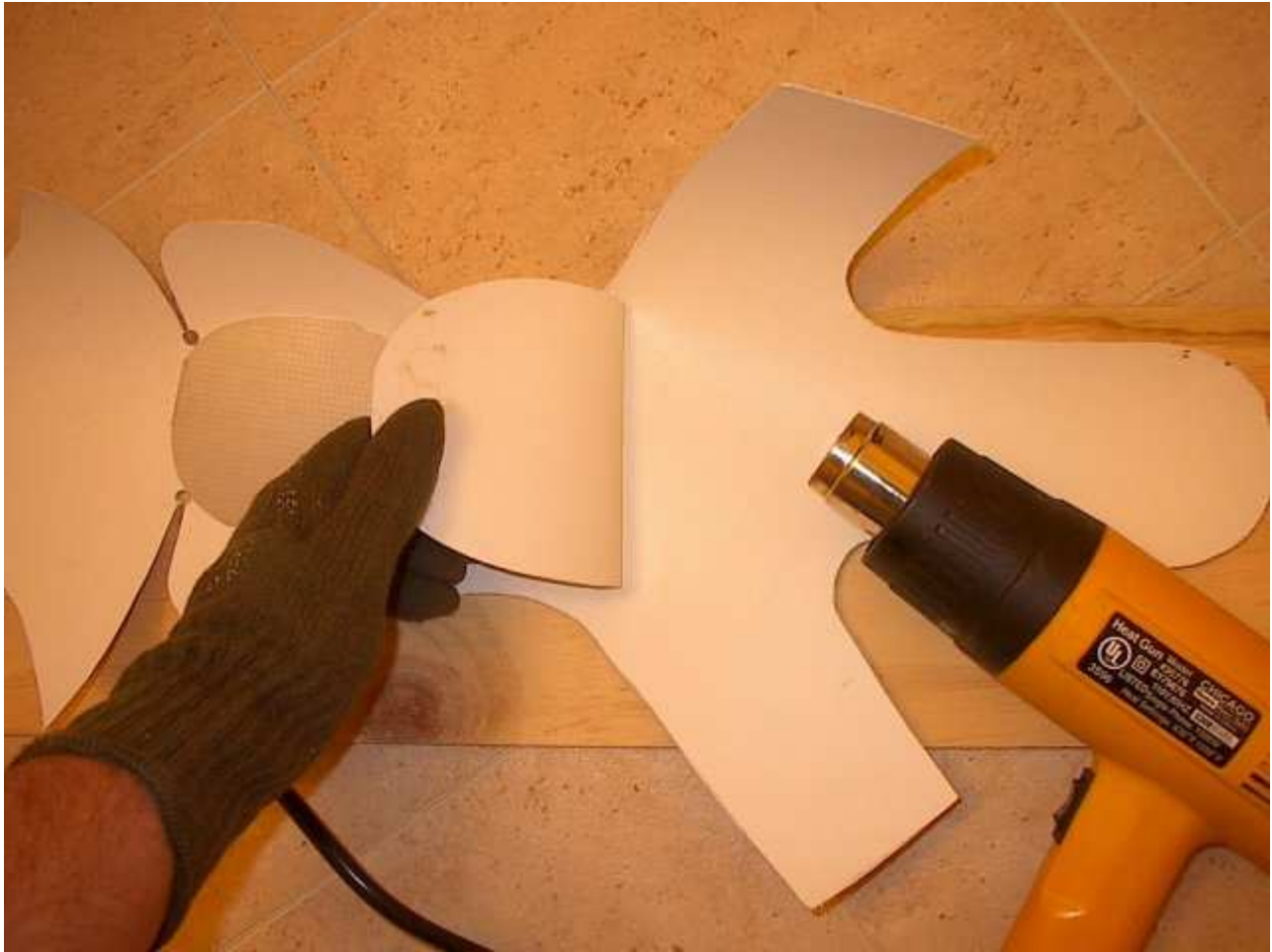
The doubler welded to the binding.
