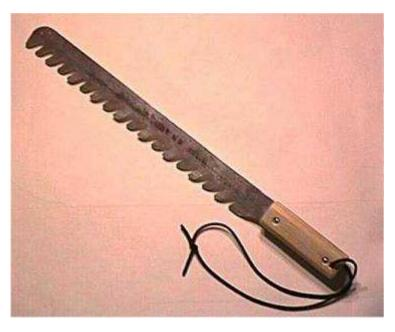
One 'weakness' in this design is that the Scouts seem to like using the saws as a pry bar to try and move snow blocks. Being aluminum, they do bend (but can be bent back into something fairly straight without noticeable damage).
