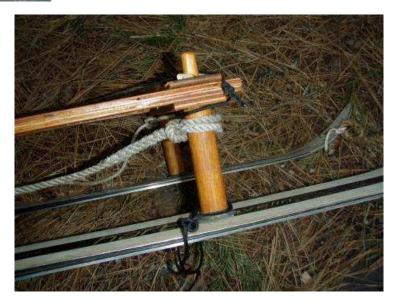
The sled itself tows very easily. The rear control line should be used by your buddy on any slopes as the sled will slide past you! It has at least 4" of ground clearance and flexes making it easy to get past humps and bumps in the snow track.
