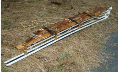
The para cord X-braces keep the sled rigid and support your gear bags! We used 1/4" ply scraps & an old broom handle for the wood. Note the lashing line tied to each vertical support with para cord tie lines to secure your gear bags. This example uses a simple over-the-shoulder towing harness but can be equipped with any of the rigid pole examples discussed on this page.
