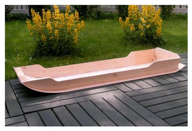
I suspect if you built one of these of ½" plywood and clear grained pine, you could improve the durability by applying either a coat of epoxy or a layer of glass and epoxy to make it tougher.
